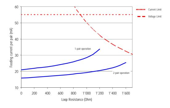
Figure 4-3 shows powering reach for single 1-pair and 2-pair regenerators under the assumption that the NTU is locally powered:
