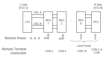
Figure 4-2: Cascading and addressing regenerators
