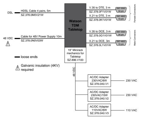
Figure 10-2: Tabletop cables and mechanics
