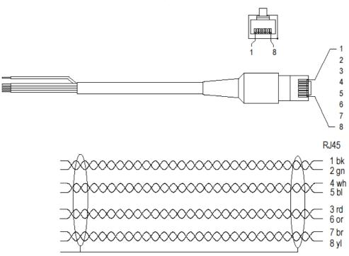
Figure 10-3: DSL Cable, 4 pairs, 5m, open end
