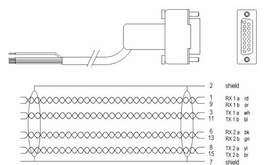
Figure 10-4: Cable 2 x E1, 5 m
