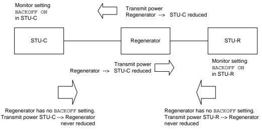
Figure 3-2: Power backoff with regenerator
