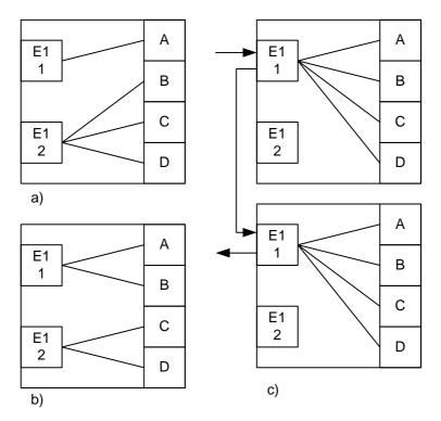
Figure 3-16: Examples of Multipoint Configuration
