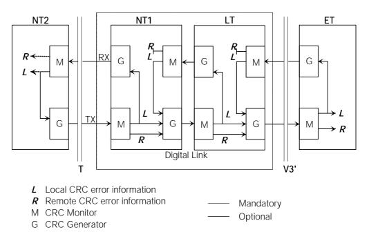
Figure 3-12: Digital Link with CRC Processing in the LT and NT1
