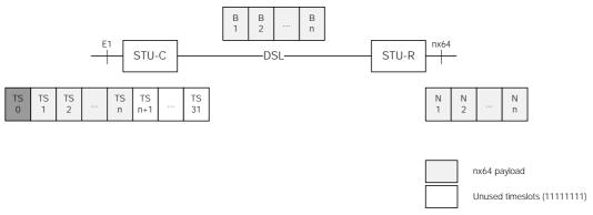
Figure 3-14: Mixed mode mapping
