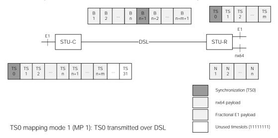
Figure 3-15: Mixed Mode multiservice mapping
