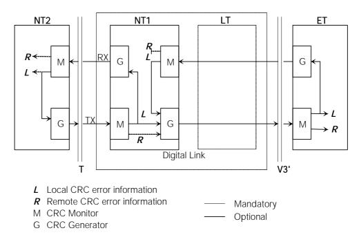
Figure 3-11: Digital Link with CRC Processing in the NT1
