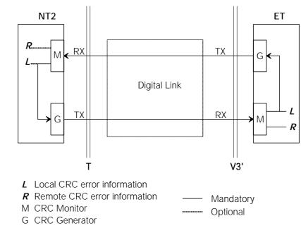
Figure 3-10: Digital Link without CRC Processing
